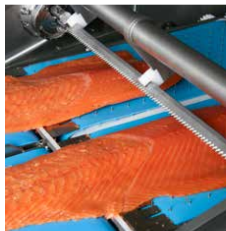
D-cut slicing: 10° – longer slices
