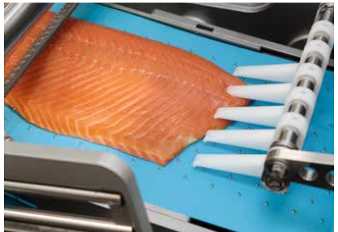
For extra support, a product holder fixes the end of the fillet on the spike belt to keep it stable during the final cuts
