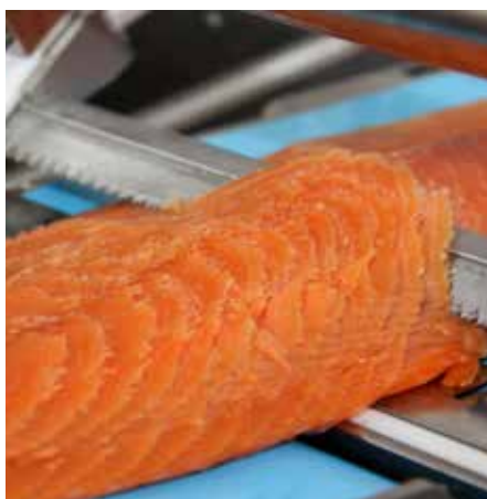
D-cut slicing: 18° – standard slices
