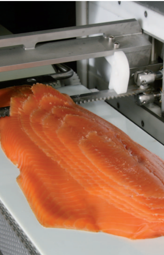
The slicing process on MSC 650-45
