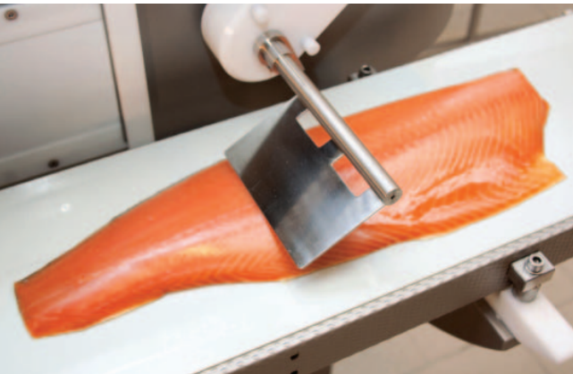
Fillet measurer for optimized slicing on MSC 650-45
